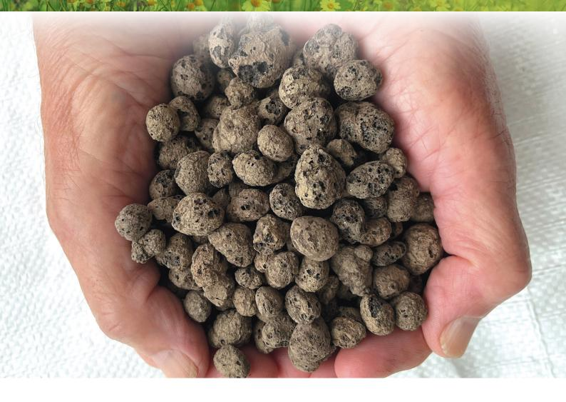
Leca® is a highly durable lightweight aggregate, which is produced in the form of a round shaped hollow clay pellet with a ceramic resistant exterior skin and a porous, lightweight, interior nucleus. Simply put, Leca® is a super lightweight, inert and non-combustible aggregate.
