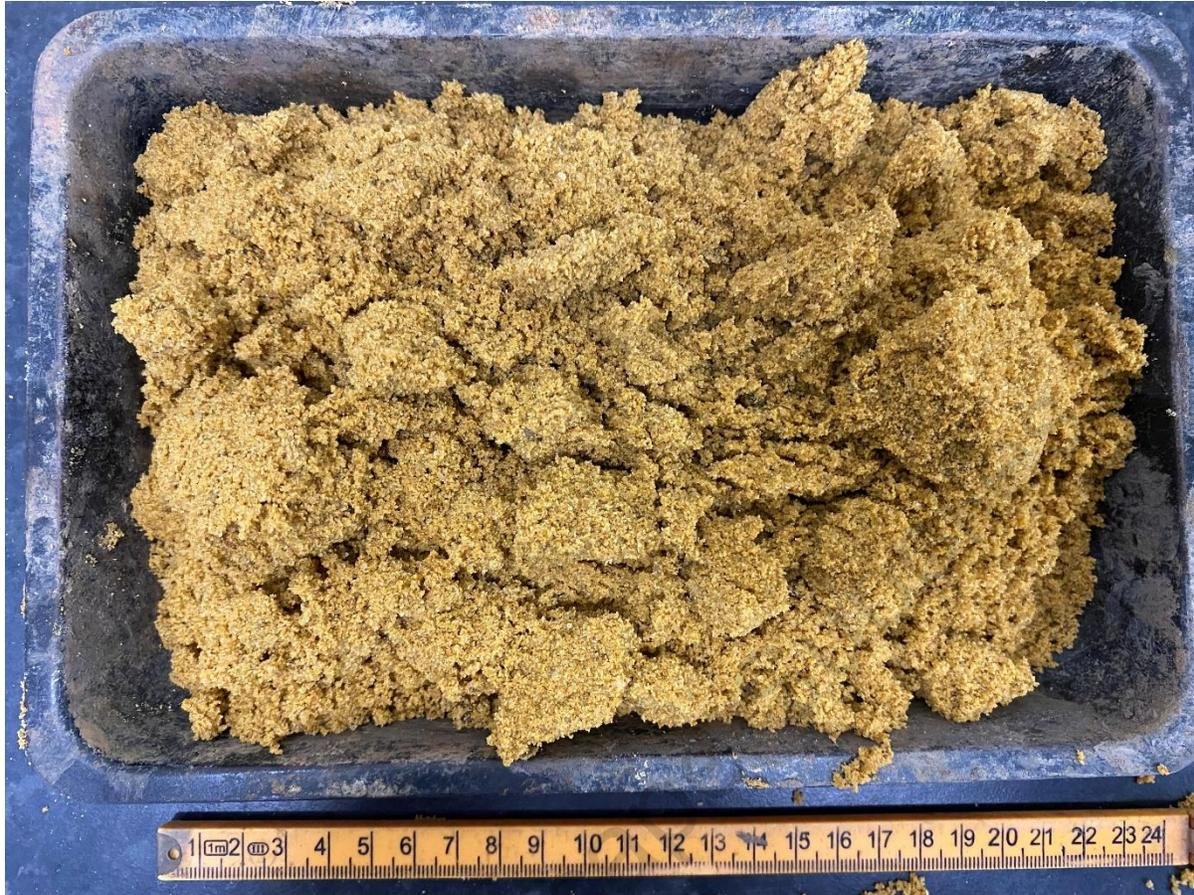
*Plate 1: Medium / Coarse Washed Silica Sand (D) Sample*
